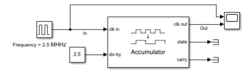
The period of the incoming pulse at the  ${\bf clk}$  in port is  ${\bf 4e-7}$  s. So, the incoming signal has a frequency of  ${\bf 2.5}$  MHz. The div-by value is set at  ${\bf 2.5}$ .
