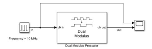
The period of the incoming pulse at the **clk in** port is 1e-7 s. So, the incoming signal has a frequency of 10 MHz. The **Program counter value**, **Prescaler divider value**, and **Swallow counter value** are 4, 1, and 1, respectively. The effective clock divider value of the dual modulus prescaler is 5.
