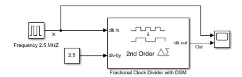
The period of the incoming pulse at the  $clk\ in\$ port is  $4e-7\$ s. So, the incoming signal has a frequency of  $2.5\$ MHz. The div-by value is set at 2.5. The clock divider uses a second order delta sigma modulator.
