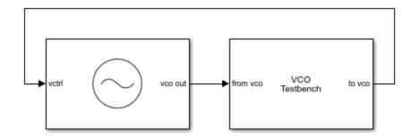
The testbench is set to measure the **Kvco and Fo** metric of the VCO in **Measurement** option. **Range of control voltage (V)** provided to the input of VCO is set to [1 10].
