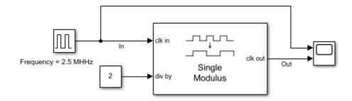
The period of the incoming pulse at the **clk in** port is 4e-7 s. So, the incoming signal has a frequency of 2.5 MHz. The div-by value is set at 2.
