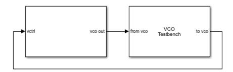
The voltage sensitivity of the VCO is set to 1.25e6 Hz, and the free running frequency is 2e9 Hz.
