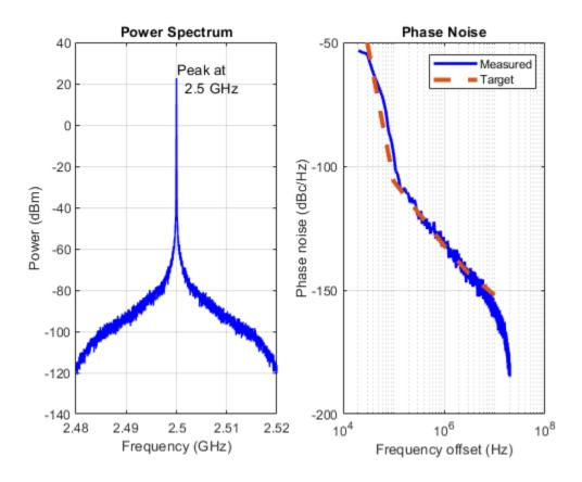
The operating frequency matches the predicted frequency  $2.5\ \text{GHz}$ . The measured phase noise profile also matches the target profile.
